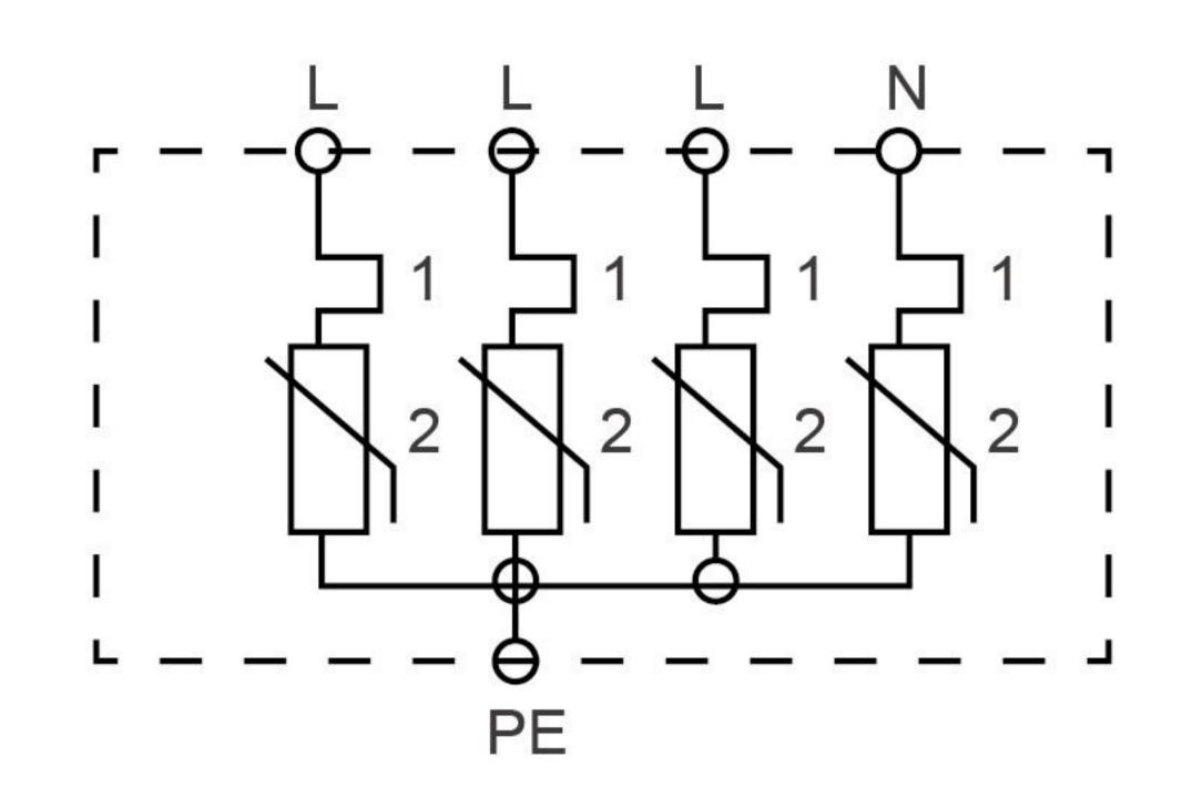
Figure 2 Note: 1.Thermal failure release 2.Varistor
